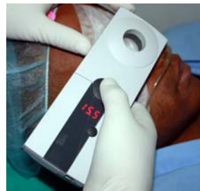
Telemetry pressure reader
